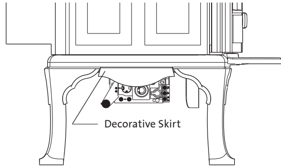
Figure 15. Remove the valve skirt for better access.
